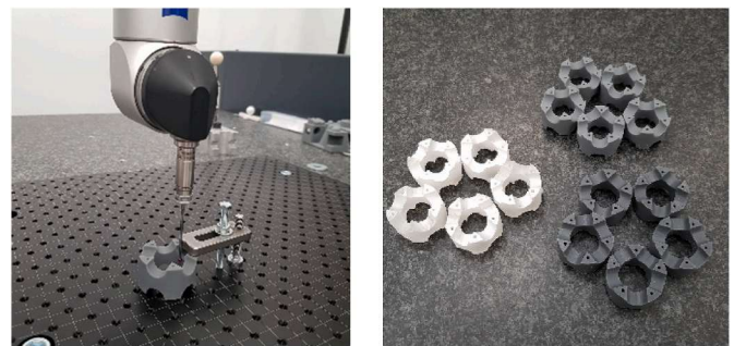
Fig. 5. On the left measurement with the use of Zeiss Eclipse contact CMM, on the right rings from various resins.
