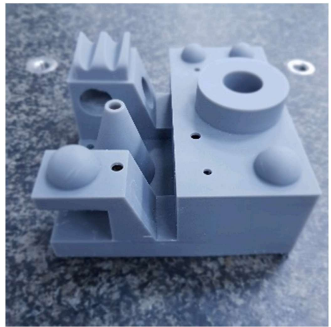
Fig. 8. A special standard for testing the regularities of SLA printing.
